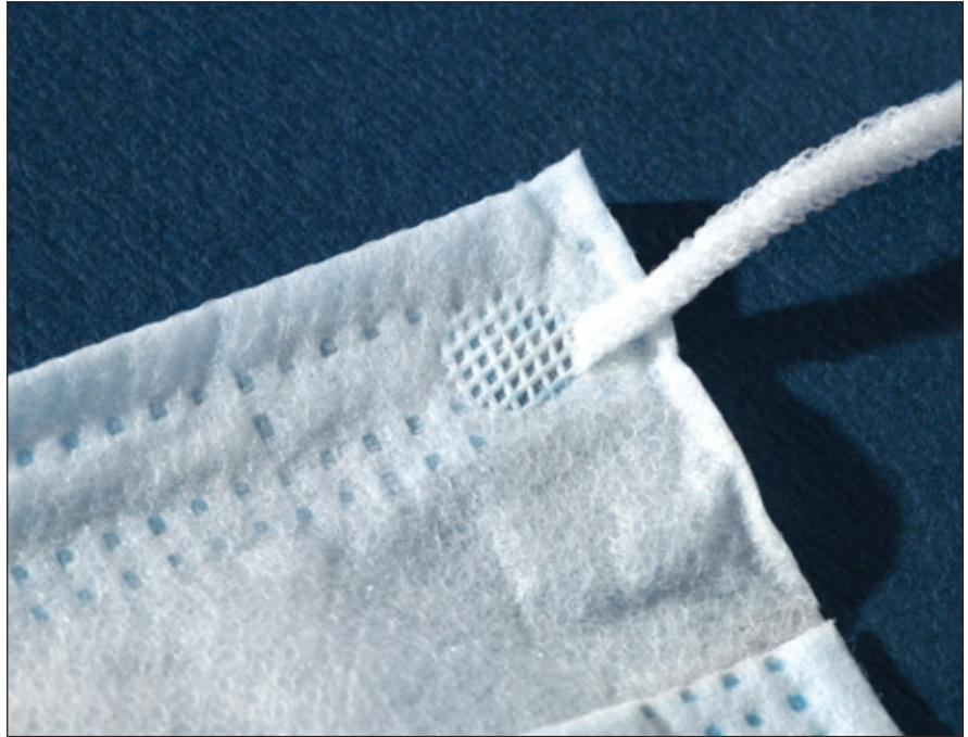
Ultrasonic welds strongly bond even small items like the ties on a disposable surgical mask at a fraction of the cost of stitchery or glue and can be used immediately. (Credit: Emerson)
